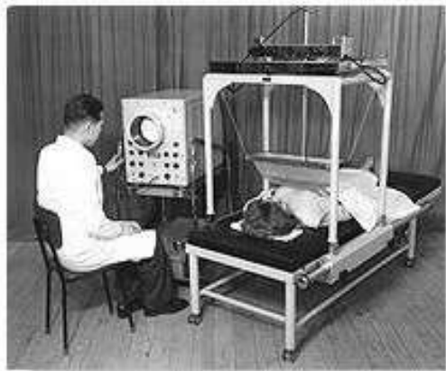
The water-bag B-mode scanning system, the SSD-1, from Aloka in 1960
