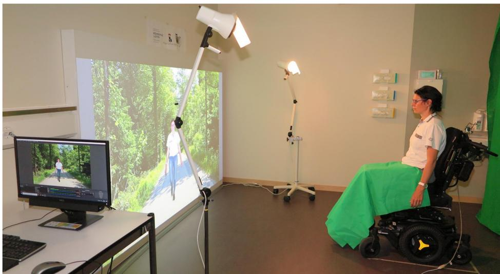
**Figure 1:** Clinical setting of virtual walking: The imagination of walking is realized by projecting the upper body of the patient merged on «walking legs» by computer technique. The wheelchair used in this setting provides an alternating side to side tilting to simulate the movement of the pelvis for a more authentic walking impression.
